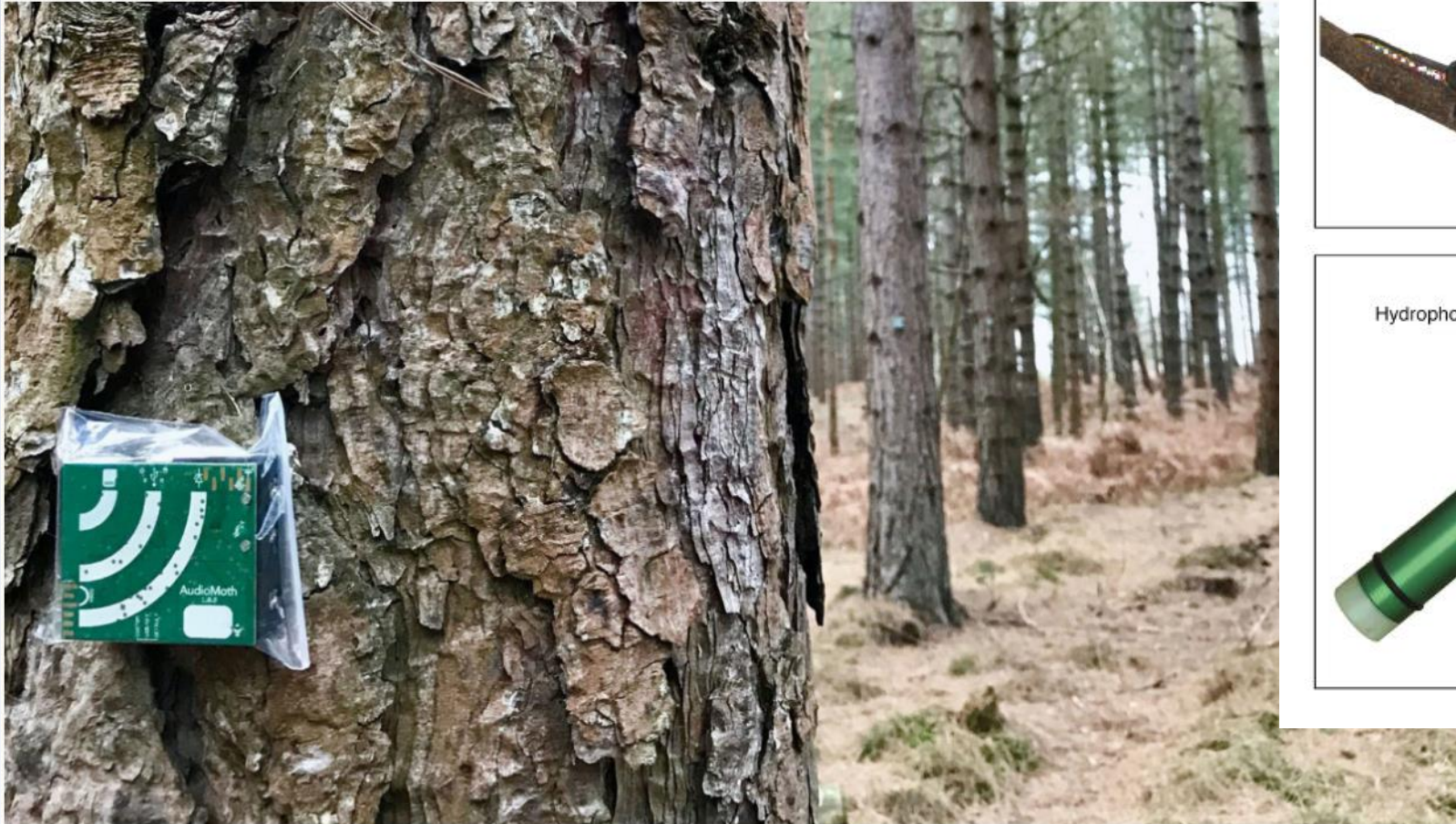
The AudioMoth recording device in New Forest National Park, in the U.K., where it is searching for sounds of the New Forest cicada. COURTESY OF ALEX ROGERS
